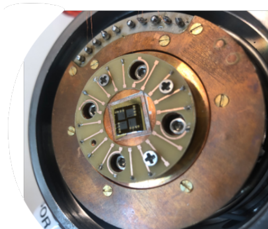
Figure 1: An image of an electrically gated chip that host various dipolar polariton devices based on gated GaAs waveguide photonic hetero-structures.
