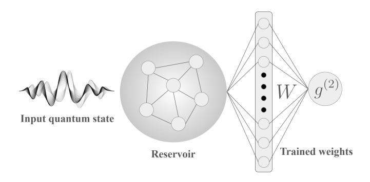
Figure 1: The reservoir is made up of randomly connected nodes. It receives the quantum input state and transforms the inputs into a high-dimensional space. The outputs of the reservoir are then trained by a fully connected linear layer.
