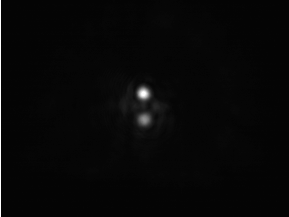
Figure 1: Momentum space picture of the probe signal and its idler after filtering out the pump signal.
